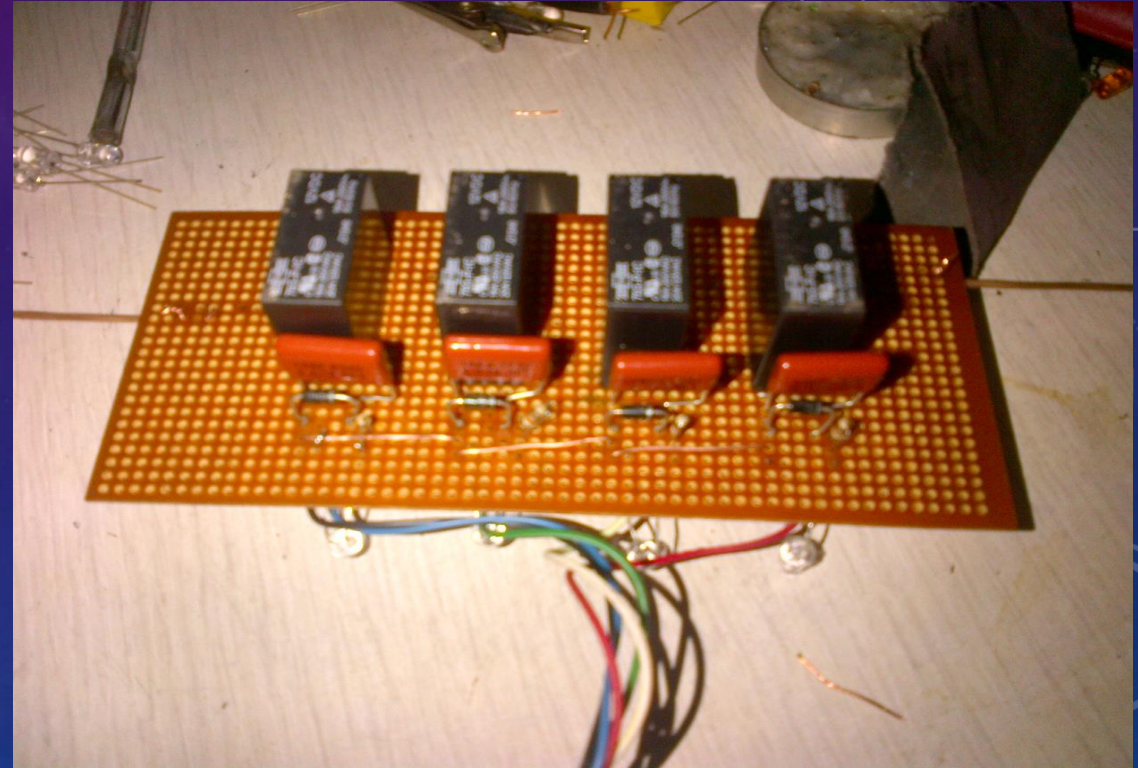
SPDT relay, rated max 20A @250V with a 12-volt coil
