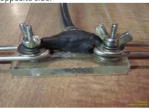
To tune the antenna for minimum SWR simply loosen the wing nuts and slide the antenna elements in or out as needed. Keep in mind that changes made to one band will affect the other band. For example if you shorten the 2 meter length then you also shorten the 70 cm length. Some fine tuning by again trimming either the 2 meter or 70 cm sections may be done if desired but this should not be needed.
